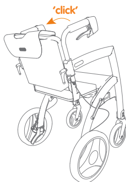
Figure 42: Click the backrest into the guide rails.
