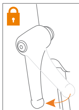
Figure 45: Tighten the adjustment handles.
